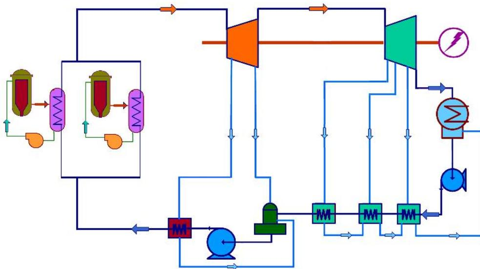
Fig. 1 - Simplified Schematic Diagram of the HTR-PM Demonstration Power Plant
